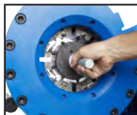
Quick Change Die Tool KCQCT-HS54
