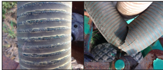
PVC Hose cracking due to UV exposure
